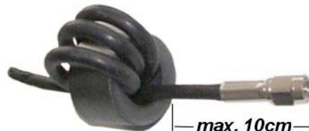
Figure 5: Installing the toroid on the antenna cable
